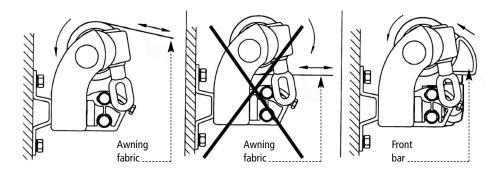
Do not continue unrolling the material once the arms are fully extended. The material should remain taut. Note: the arms will have a slight bend when the awning is fully extended for added stability.
