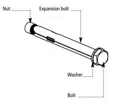
Insert the expansion bolts through the wall bracket, and then plug the expansion bolts into the drilled holes. Check to ensure all wall brackets lie on same horizontal line before ensuring all nuts are securely tightened. Check the brackets are tightly fitted against the wall before attaching the awning. If any movement occurs when attaching the awning, remove the awning from the wall brackets, inspect the wall brackets for movement, and further tighten the nuts if necessary.
