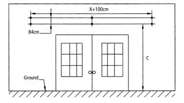
Ensure the drill holes are located in brickwork or concrete. Do not drill into mortar, this will not provide adequate strength to hold the awning.
