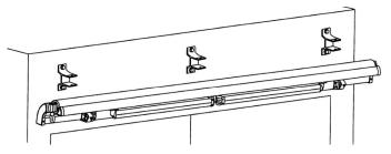
Remove the bolts on the front of the wall brackets. Raise the awning into position and gently locate the square torsion bar to the wall brackets and then lock into place by replacing the nuts and bolts. Tighten the nuts to ensure the awning is attached to wall brackets securely.
