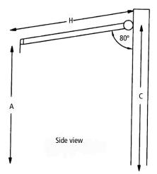
**Note:** Always ensure there is sufficient headroom and that any doors or windows can open fully when the awning is fully extended. 20cm clearance above door frames is recommended. The recommended installation height is between 2.5m - 3.5m.
