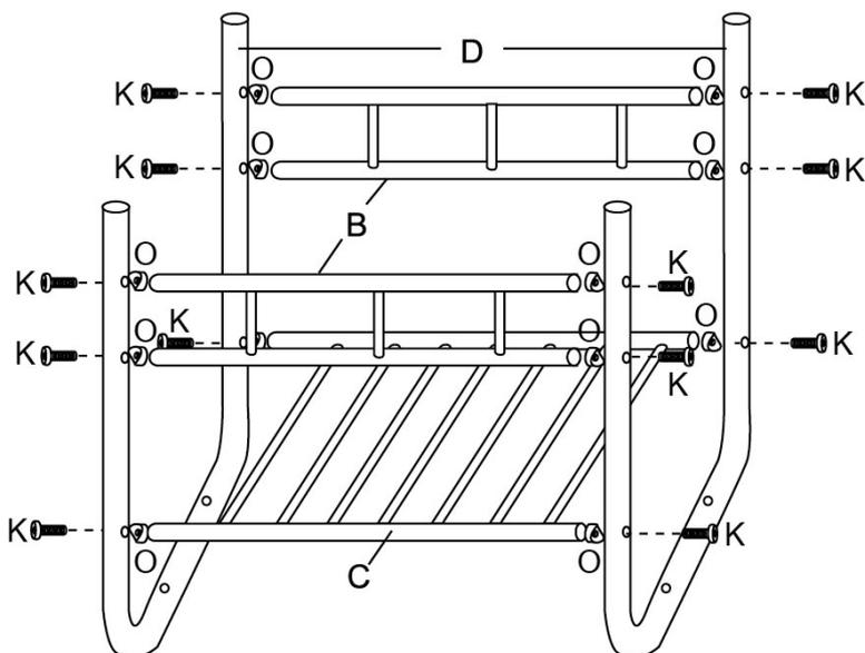
Connect 2x piece D to 2x piece B and 1x C using screws K x12 and washers O x12 as shown with the Allen keys (P) provided.
