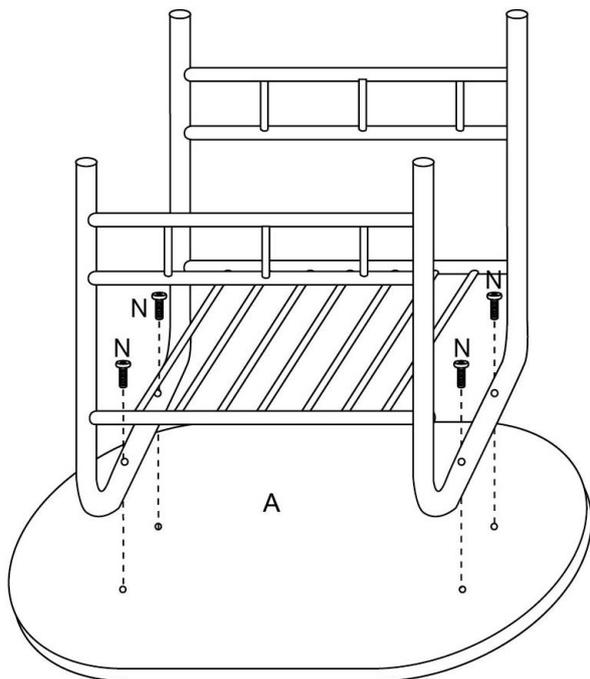
Fit part A x1 to assembled pieces using screws N (x4) as shown.
