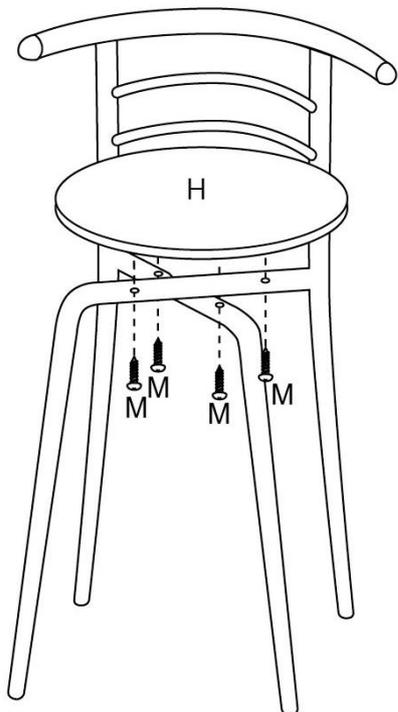
Using screws M (x4) connect leg assembly with seat H (x1).
