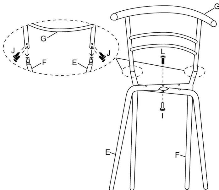
Connect part G (x1) part E (x1) and F (x1) using screw L (x1) and nut I (x1) as shown. Where indicated by a circle connect G with F on one side and G with E on the other side using 2x screw J on either side.
