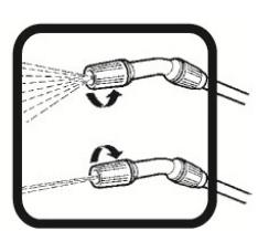
Twist nozzle to adjust flow
