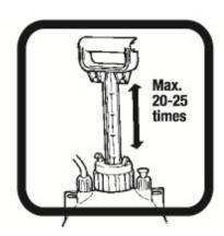
Push and pull to built pressure maximum 20-25 times.
