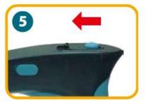
If you want to switch to Momentary Mode, slide the switch on the top of the handle forward until it clicks into place.
