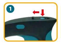
Make sure that the switch on the top of the handle is pushed forward. Press the blue button on the top of the handle then push the switch forward.
