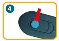
Push the blue button on the top of the handle to release the object.
