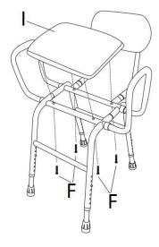
Put part # I (Seat) on top of the Front and Back frame. Insert part # F(Screws) with a screwdriver (not included) to tighten the Seat.
