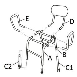
**Note:** The height of the stool can be adjusted by pressing the two buttons on each foot pieces. Make sure the stool is stable after each height adjustment.
