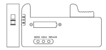
**Note:** A fully charged 1.2V rechargeable battery will only light the **RED** and **YELLOW** LEDs. This is normal. Make sure the polarity is correct when testing, otherwise, no LED will light up giving a false reading.
