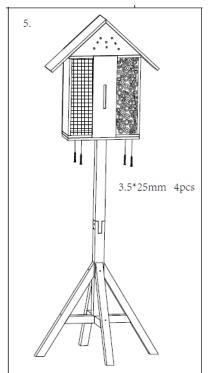
Step 5 Fix insect house to board with 4x 25mm screws as shown.
