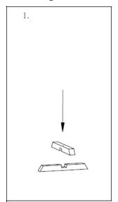
**Step 1** Slot together parts 6 and 7 as shown.
