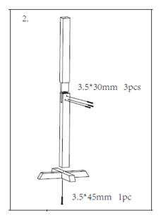
**Step 2**Connect the base with 45mm screw as shown. Connect
