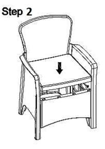
Place seat pad on top. Align pegs with slots.
