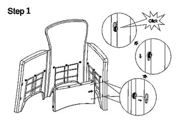
Fold side panels in by 90° and connect with front panel.
