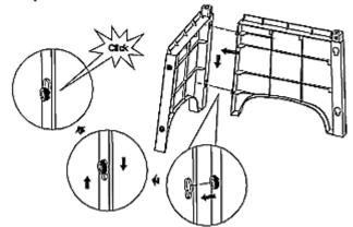
Align pegs with slots, insert pegs into slots and push down until it clicks and locks.
