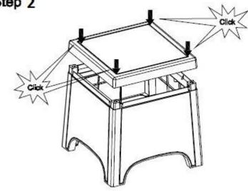
Align pegs with slots, insert pegs into slots and push down where indicated until it clicks and locks.
