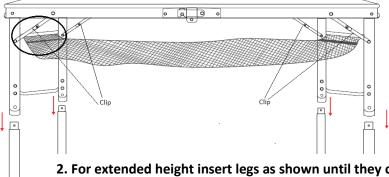
2. For extended height insert legs as shown until they click in position. Ensure all four clips are fully extended and in place – see illustration.
