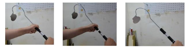
Connect both parts, rotate until tightened then adjust the pole length as required
