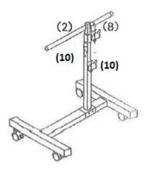
3. Insert (2) into (8) (1) and twist tightly with screw handle(10)
