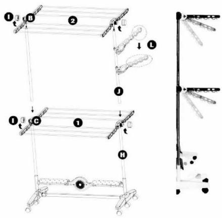
STEP 5: Slide the vertical tubes (J) into the vertical base tubes (H).
