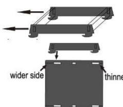
1. Connect both A parts with B parts in rectangular sequence (like in a photo). Make sure both A parts bottom hooks face in the same direction.
