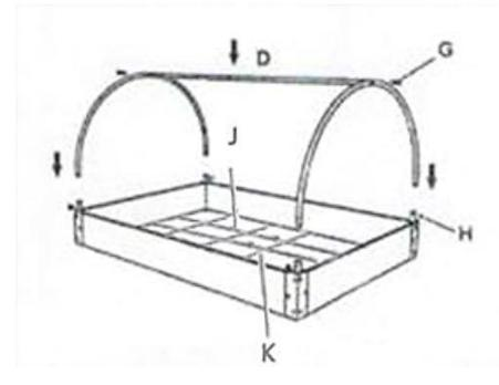
Assemble frame (D & G) and insert into holes in the base (H) as shown.
