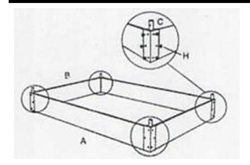
Assemble frame (A & B) connect with corner pieces (C) using bolts (H) where indicated.
