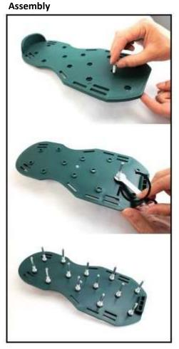
**Step One** Insert spikes into holes and tigthen with spanner Turn clockwise.
