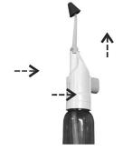
2. To remove the nozzle from the device press the release button and pull nozzle from it at the same time.
