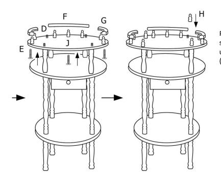
Place part J on top. Insert screw E (x9) to screw in place knobs D (x9) from underneath. Then push parts G (x2) and F (x1) in place.
