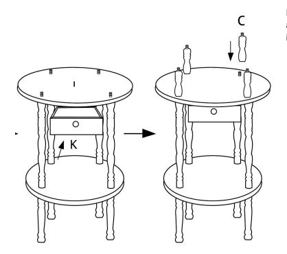
Place part I on top of the assembly and attach parts C 4x.Part K (drawer) is inserted underneath part J.
