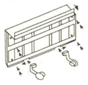
Wall mount dispenser. Fit fixings provided through the pre-drilled holes. To fit to tiles use pads supplied. Attach bottom roll holders as shown.
