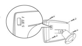
Step3: Replace battery compartment cover, screw it back into position and make sure is properly sealed.
