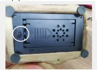
Push the battery case in the direction of the arrow and open it to replace batteries as shown.
