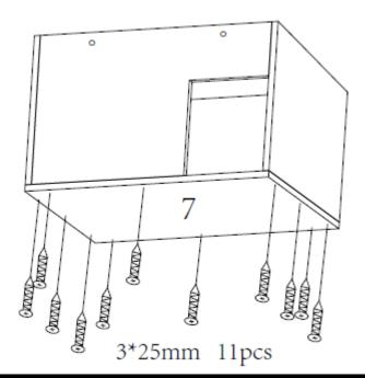
Fix 1pc of base to the assembly using 11pc of 3\*25mm screws
