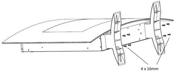
Eight 4\*16mm screws are used to fix the feet to the product, as shown in the picture on the previous page. Always use your appliance with feet fixed.
