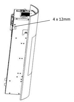
Align the brackets on the back of the electric heater with the slot in the wall bracket as shown.
