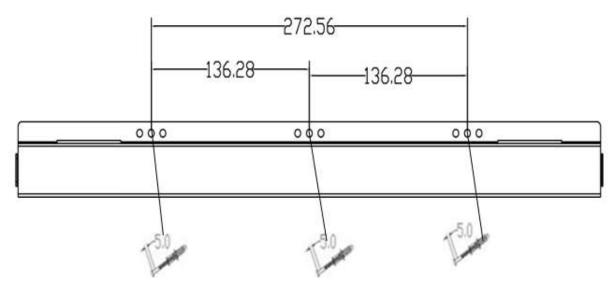
First, fix the three dowels to the wall according to the distances shown in the picture below, then drive the three 4\*45mm screws into the wall mounting bracket and into the dowels that have been fixed to the wall.
