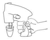
2. Pump water through the tube by pulling the trigger for 15 seconds.
