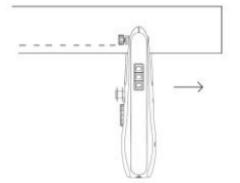
4. Hold the handle of the sewing machine and operate the power switch with your thumb.
