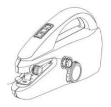
3.Draw the thread from the spool through the thread guide and pull the thread through the tension control. Do not wrap the thread around the tension control. Note: To loosen the tension control turn the dial clockwise.
