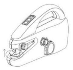
1.Start by raising the needle arm to Its highest point by turning the rotary wheel in either direction.
