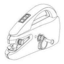
2.Remove the bobbin pin and place the spool of thread on the bobbin and begin to thread through the thread guide to the tension control. Note: The spring must be in place before installing the bobbin.
