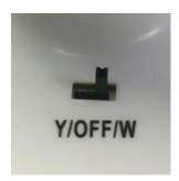
Turn the lamp on at the **switch**. Select Y for yellow light or W for white light. Select OFF to turn off the light.
