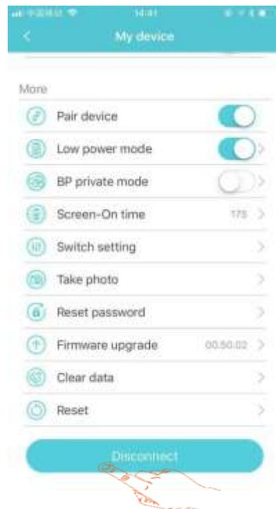
The watch interface shows a disconnecting with smartphone
