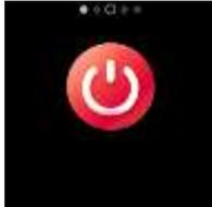
In the Power interface, long press the screen to shut down (see icon).
