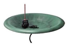
3. Insert the pump housing pipe into the hole on top of the pump. Rotate the nut and washer on the pipe until they are tight at the top of the pump housing. Ensure that the rectangular guide is flush with the raised areas. The bottom of the pump should be flat against the base of the pump housing.
