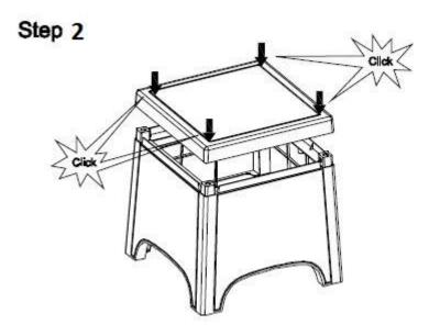
Align pegs with slots, insert pegs into slots and push down where indicated until it clicks and locks.
