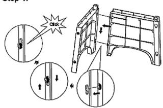
Align pegs with slots, insert pegs into slots and push down until it clicks and locks.
