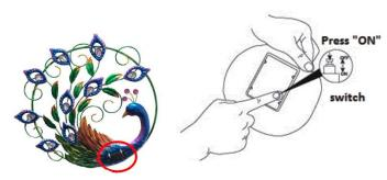
NOTE: The solar panel is located on the body of the peacock as shown where circled.
