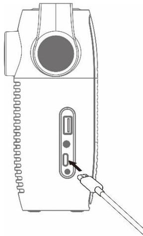
2. Connect the other end of the Type-C cable to a power outlet, using a USB power adapter. You can also charge the battery by connecting to a computer's USB port. Charging indicator shows the battery charging.
