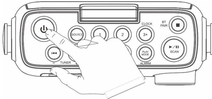
4. In standby mode Press and hold the POWER
