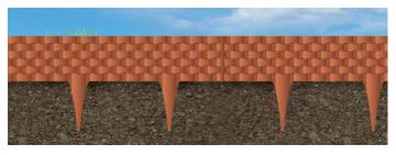
Insert 1 panel as required. Then line up another panel so the two interlock as you are pushing the second panel into the ground.
