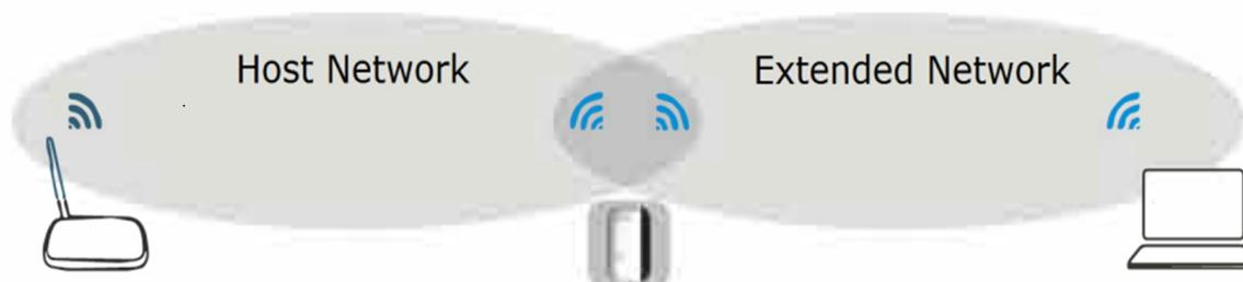
The repeater Wi-fi booster to the end of the host network's SSID and uses the same Wi-Fi password.
