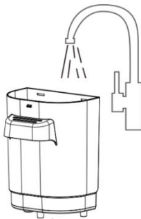
5. Rinse the sewage tank, dry it in the shade and then reinstall it.
