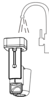
6. Clean the buoy bracket, dry it in the shade and then reinstall it.
