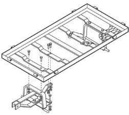
3. Attach the front axle support (9) to the trolley base (10) using 8x20mm carriage support bolts (260, washers (21) and locking nuts (22) – see left.
