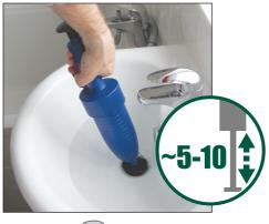
When clearing a sink, please ensure the overflow is covered A and the U bend is supported B it is recommended that there is at least 7cm of water in the sink C.
