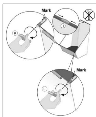
7. Attach the hopper crossbar (d) to the handle and assembled hopper ensuring the hopper rods and the handle click securely into place with the clips on the hopper crossbar (d). Ensure this is fitted correctly with the hopper rods clipping into the hopper crossbar (d) from above. If assembled incorrectly, the hopper can detach during use.
