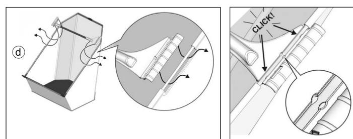
8. Press together the holes and pins at the top of the brushes (n) to form 4 sets.
