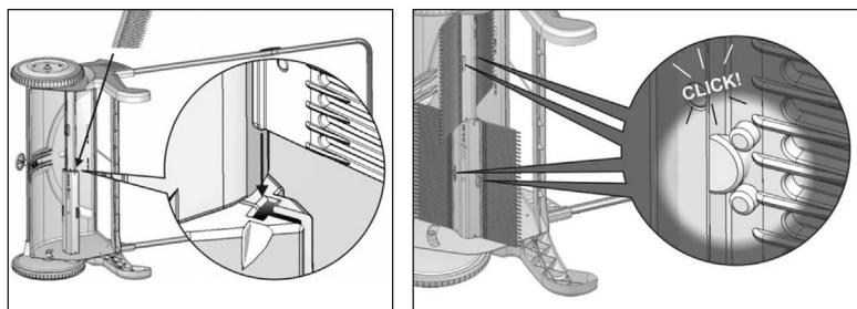
10. Clip the assembled hopper into position on the handle and slot the connectors into the recesses on the sweeper body (m).
