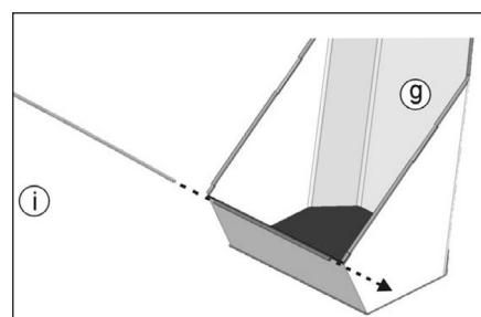
6. Connect the hopper frame side rods (h) together using top frame connector (j). Connect the hopper frame base rod (i) to the assembled frame by connecting hopper frame connector right (k) and threaded end of hopper frame connector left (l) to the threaded ends of the hopper frame side rods (h). Connect both connectors to the hopper frame base rod (i) ensuring the shorter horizontal fitting on the connectors are facing outwards.
