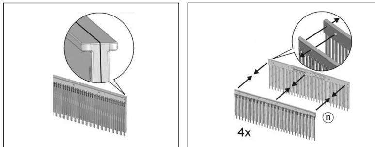
9. Hold the assembled brush sets together and slide each set into the grooves on the rotor until each set clicks into place.
