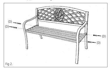
• After finished above steps, fully tighten all nuts and attach end caps. The bench is now ready for use.
