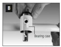
Slide the bearings and steel rod into the bearing case.
