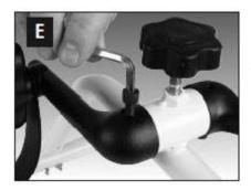
Push the second pedal onto the steel rod and tighten bolt with the Allen key. Repeat steps A to E to assemble the handlebar pedals.
