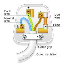
The diagram shows the key features of a correctly wired three-pin mains plug.
