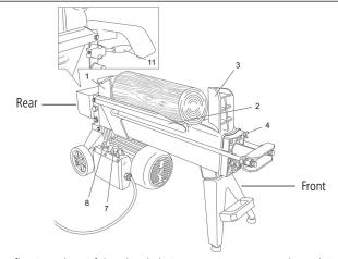
Air must flow in and out of the oil tank during operation to prevent the seals in the hydraulic system from rupturing.
