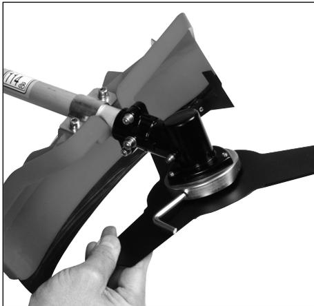
3. Attach the spacer, end cap blade and locking nut and with one hand hold the Allen key and the other hand tighten the locking nut in a clockwise rotation using the spark plug socket.
