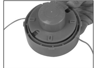
Line up the slot on the bottom cap with the hook on the housing, press the cap against the housing and twist in an anti-clockwise motion to secure the cap to the spool housing.
