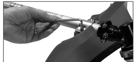
5. Align the holes in the drive shaft and insert the 5mm Allen key through both holes.
