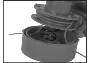
While holding the spool against the housing, pull the line ends to release them from both slots. You don't want the line to be secure in these notches when in use as the line won't feed through when you press the bump start button.
