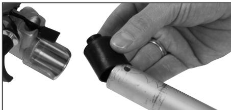
3. Connect your new drive shaft in the same joint connection, making sure the gears interlink correctly (you may need to twist the drive shaft a couple of times for drive shaft to lock into place), then tighten the knob bolt on the drive shaft securely.
