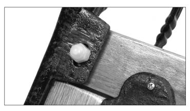
Using the strap place over the 5 marked points you have made on all five wooden slats. Using a Phillips screwdriver and 5 x wood screws attach the strap to the wooden slats.
