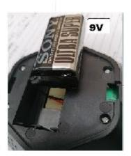
Ensure red and black wires run under the connector as shown above.
