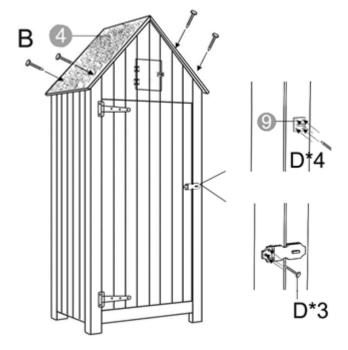
Step 6: Attach the Roof Part 4 to the main frame by using Part B Screws.
