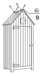
Step 7: Attach the Wooden Middle Bar Part 7 across the middle of the roof with 4x Part 7 Screws.
