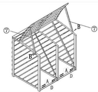
Fit the 2 wooden holders (7) using 2x screws B.
