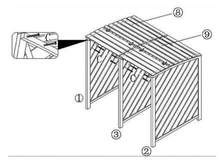
Fix the 2 roof panels (8 and 9) to the left (1), middle (3) and right panel (2) using 8x screws C.
