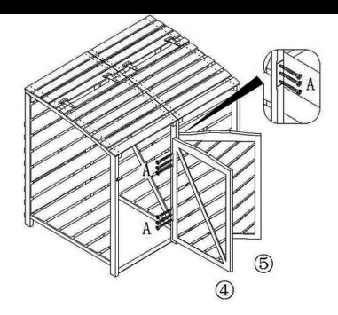
Fit left door (4) and right door (5) to the front of the unit using 12x screws A where shown.
