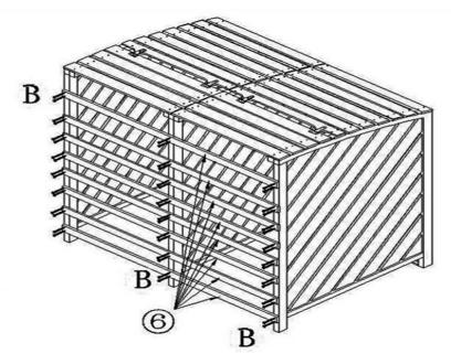
Where indicated by arrows fit 8x wooden lathes (6) using 48x screws B.
