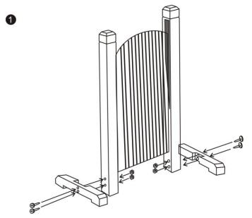
Assemble wooden stands with the nut and bolts provided as shown.
