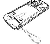
Replacing the battery cover
