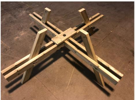
1) Take both leg assembly frames and slot them together as shown in the picture above.
