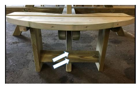
5) Fasten two 3" screws through the wooden support and into the leg of the picnic table where the arrows indicate. Repeat for the other three seats.
