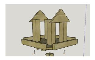
Put the roof panels in place so the top points of the detailed fascia line up screw the fascia together using 1 x 60 mm screw in each.
