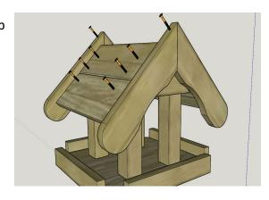
3. Finally position the house on top of the stand post centrally and screw in place using 2 x 70mm screws as shown And screw the cap strip on to the top of the roof join using 2 x 35mm screws.
