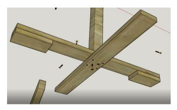
3. Position the 4 x angled supports onto the base, ensuing that they are flush to both the base and the post. Fix each each support using 2 x 50mm screws, one through the base and one through the post in each support.
