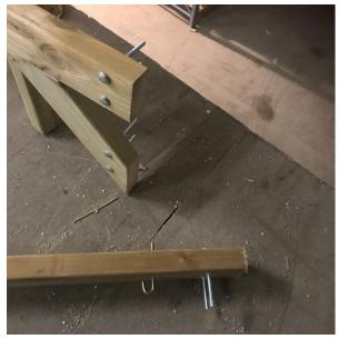
2) Take the swing sides (parts 1 &2) and place the swing hook bar (part3) on top of them, knocking the bolts through down into the swing sides. Please ensure at this stage that the cup holders on the swing sides are facing inwards. Do not tighten up the nuts yet. When knocking the bolts through if the fit is overly tight, we advise just running a 9mm drill bit through the holes again, as the wood can swell and expand with differing humidity and weather conditions during storage and transit.
