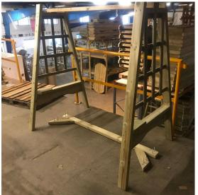
3) Next attach the rear support bar as shown in the picture, you should knock the bolts all the way through the swing sides. Try to get all the bolts lined up first rather than knocking one end fully in first, as this make it difficult to then get the other end in.
